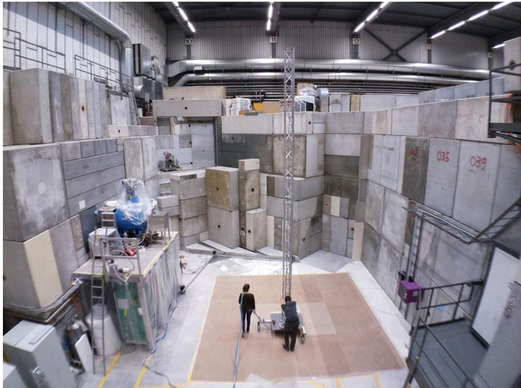
Figure 53: Area South in the UCN hall at PSI—The location of the nEDM and n2EDM experiments at PSI. The brown square outlines the foundation for the n2EDM apparatus, covered with plywood. The mapping tower is being pushed around by one person; another holds the cables. The L-piece with the string potentiometers is visible in the far end of the hall.
