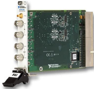
FIGURE 4.9: *National Instruments PXI-4461 module with two ADC and two DAC channels with independent timing.*
